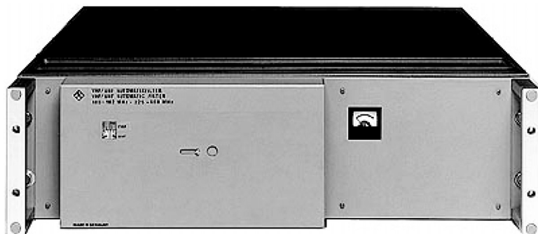
Figure 10.6 Typical cavity filter. Reproduced from Rohde and Schwarz.
